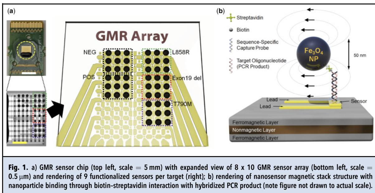
**Fig. 1.** a) GMR sensor chip (top left, scale = 5 mm) with expanded view of 8 x 10 GMR sensor array (bottom left, scale = 0.5 μm) and rendering of 9 functionalized sensors per target (right); b) rendering of nanosensor magnetic stack structure with nanoparticle binding through biotin-streptavidin interaction with hybridized PCR product (note figure not drawn to actual scale).
