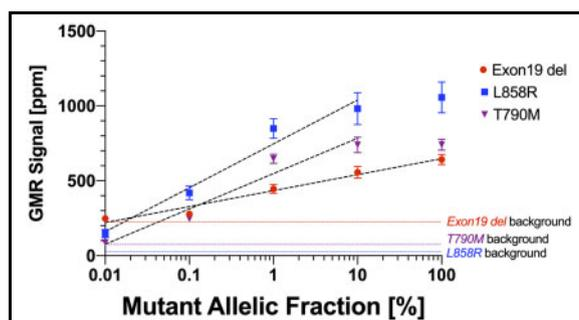
**Fig. 2.** Multiplexed GMR standard curves for Exon19 del, L858R, and T790M mutation dilution series, with total DNA weight of 30 ng. Background signal was defined as  $2\sigma$  of the median GMR signal of 0% MAF for each mutation.
